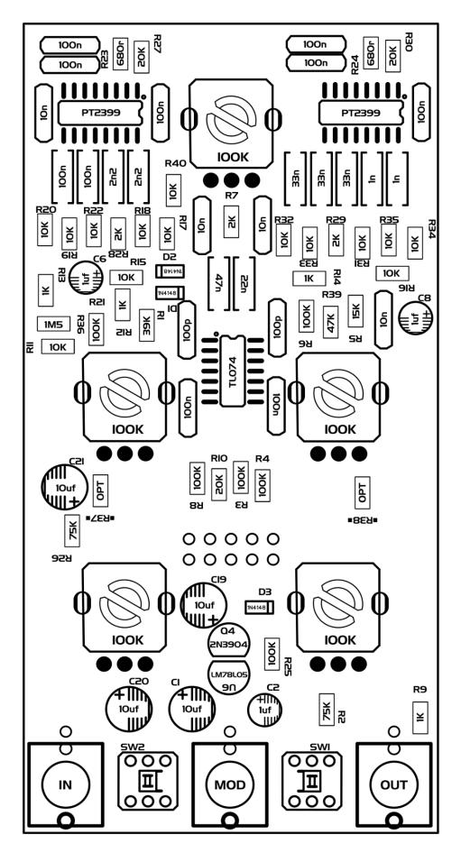
**\*OPT\*** - Optional **\*\***Buttons must be placed in specific orientation. See "Button orientation" section under step 9.
